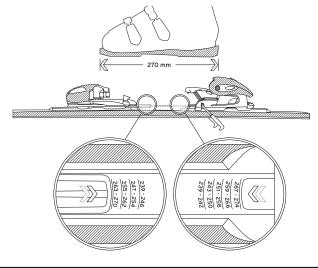
**Determine the boot sole length.** LiteRail covers boot sole lengths from 199-347 mm.
