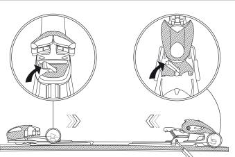
**Open toe lever,** slide toe on the base and close lever at the appropriate position.
