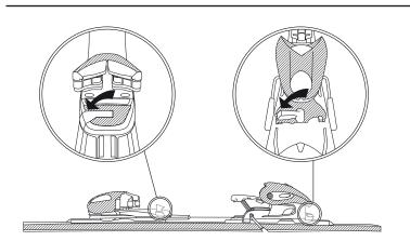
Hook brake into the heel, open the heel lever, slide heel on the base and close heel lever at appropriate position. OFF YOU GO.
