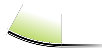
SPECTRUM 95 AND 105 has R=500 and length of the tip is 250mm
