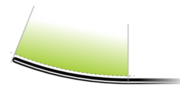
SPECTRUM 115 have R=800 mm and length of the tip is 300 mm
