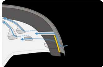
VENT STOPPERS Similar to the SCOTT Cool Plug ventilation system, the inner pads can be folded below the inner padding to unblock the top vents, thereby allowing warm air to move out of the helmet.
